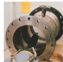
Radiographic inspection checks the integrity of welds.
