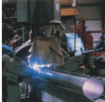
Automatic straight-seam welding using double-head, gas tungsten-arc produces pipe and tubing in sizes up to 24 inches and in continuous lengths up to 20 feet. Sizes up to 54 inches are also available, using other welding techniques.
