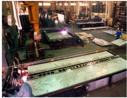
70 ft. wide clear span plate fabrication facility served by overhead cranes totaling 30 tons of lifting capacity.
