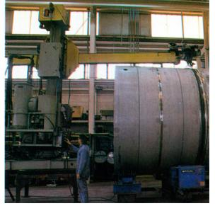
Circumferential seam welding of a large pressure vessel using a submerged-arc welding manipulator and turning rolls.
