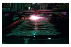
Computerized automatic plasma cutting creates multiple parts and complex shapes up to 3'' thick and as large as  $96'' \times 240''$ .
