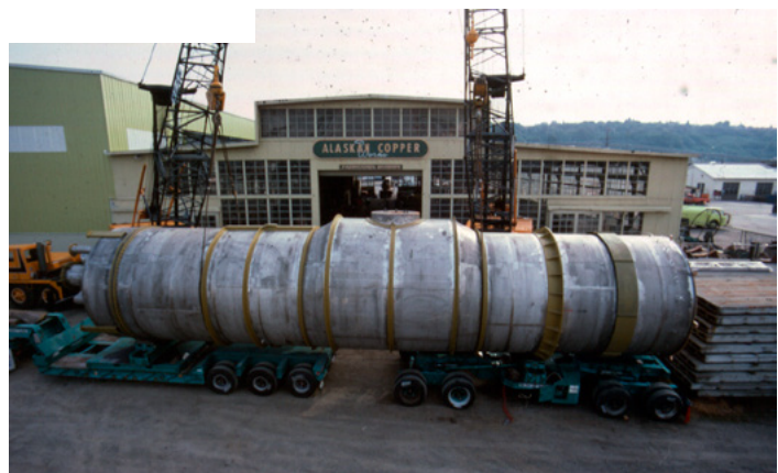
Heating element of a vapor recompression evaporator being carefully prepared for special shipment.
