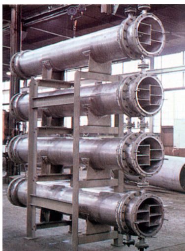
Nickel 200 8-pass, 4-shell heat exchanger.
