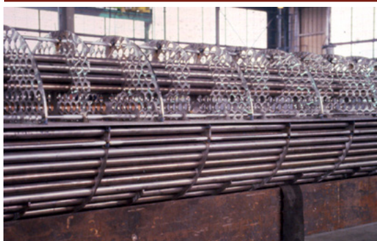
Segmental baffles used with two shellside passes.
