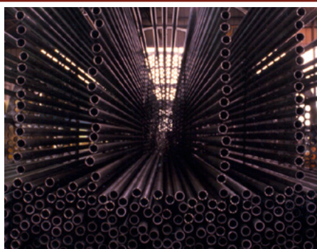
Heat exchanger partially loaded with tubes.
