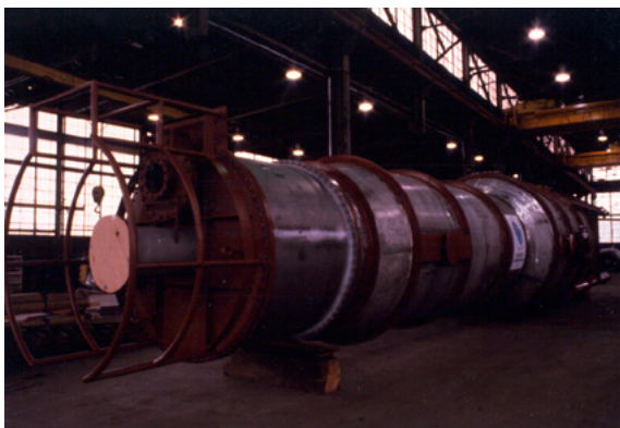
Stainless steel and titanium heat exchanger.
