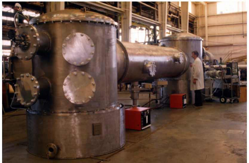
Stainless steel vacuum chamber used for free-electron laser experimentation.
