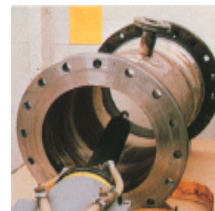
Radiographic inspection checks the integrity of welds.
