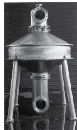
Aluminum wet pump pressure vessel used to transfer fish from a ship's hold to the dock.
