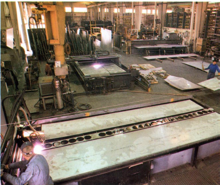
70 ft. wide clear span plate fabrication facility served by overhead cranes totaling 30 tons of lifting capacity.
