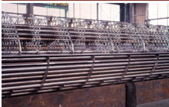
Segmental baffles used with two shellside passes.
