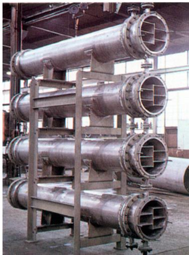
Nickel 200 8-pass, 4-shell heat exchanger.
