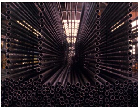
Heat exchanger partially loaded with tubes.
