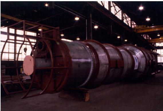
Stainless steel and titanium heat exchanger.
